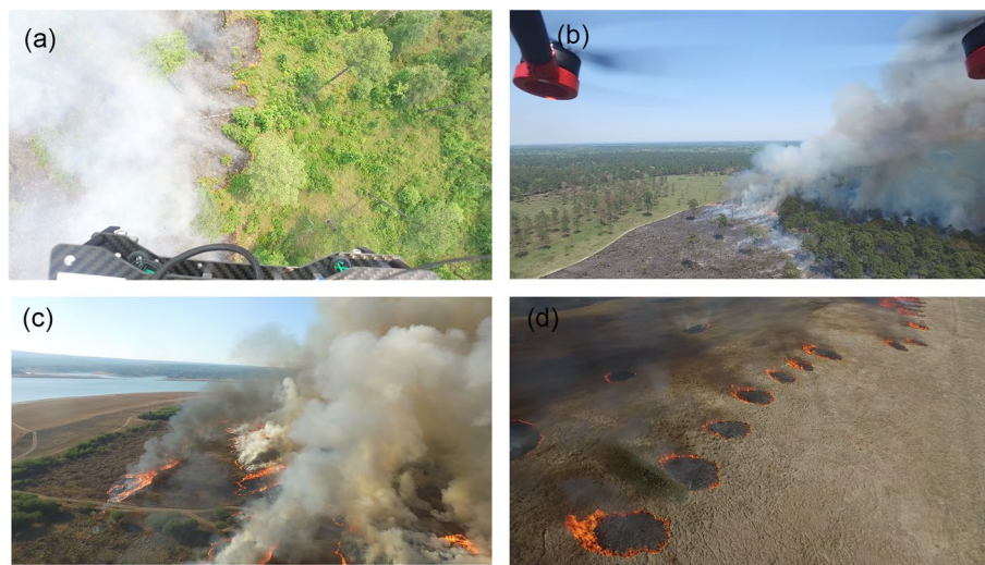
Fig. 1 Various aerial perspectives during UAS aerial ignition. a Looking straight down, with the IGNIS in view, at a longleaf pine forest burn in Vernon Parish, LA. b A recently ignited area at Cook's Branch Conservancy in Montgomery County, TX, with the two front M600 prop arms in view. c A recently ignited area along the Colorado River in Burnett County, TX. d An example of ignition drop points beginning to radiate outward during a Coastal Prairie Burn in Waller County, TX
